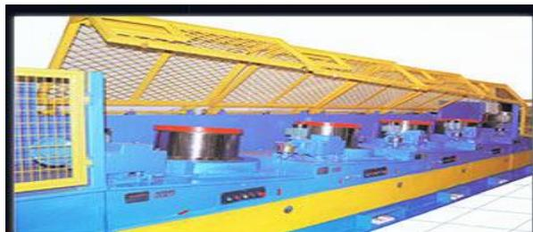
Fig. 8. A wire drawing machine [8].
