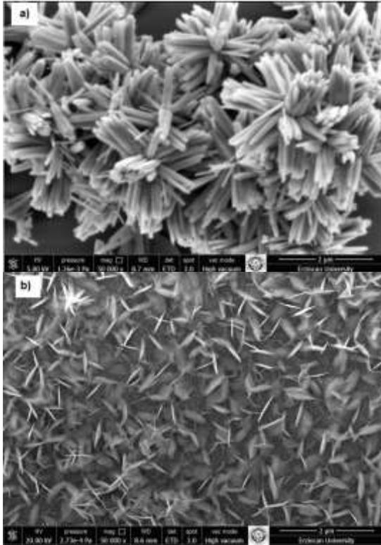
Figure 2. SEM images of the a) Zn doped CdO b) Ni doped CdO.
