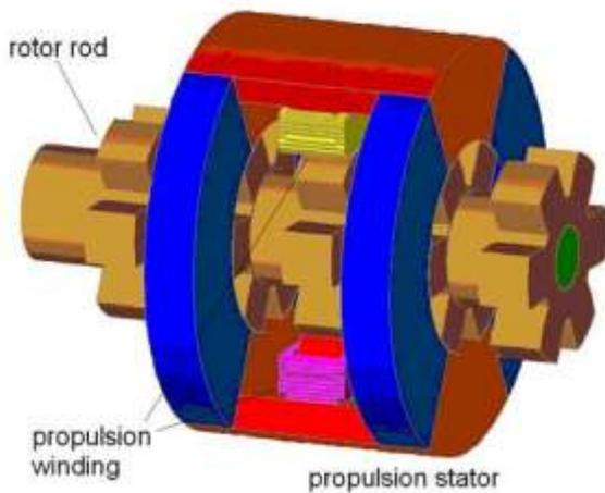
Fig.2 Structure of propulsion stator in one phase
