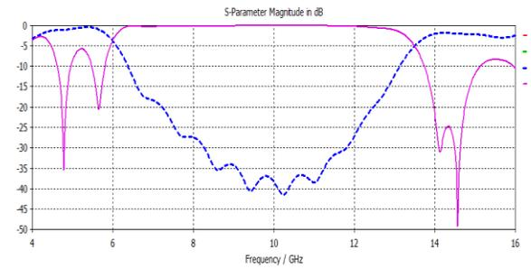
Fig. 4(b). Simulated  $S_{11}$ (solid line) and  $S_{21}$ (dotted line) for Hanning window
