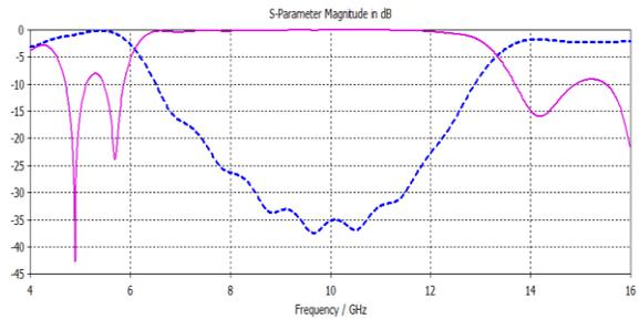
Fig. 4(f) Simulated  $S_{11}$  (solid line) and  $S_{21}$  (dotted line) for Bohman window
