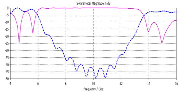
Fig. 4(e) Simulated  $S_{11}$  (solid line) and  $S_{21}$  (dotted line) for Riesz window
