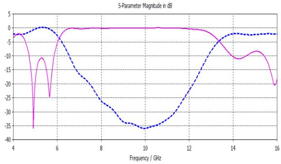
Fig. 4(d) Simulated  $S_{11}$  (solid line) and  $S_{21}$  (dotted line) for Blackmann window
