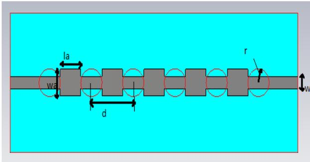
Fig.1(a) Schematic of EBG based Microstrip Filter Structure (Top View)
