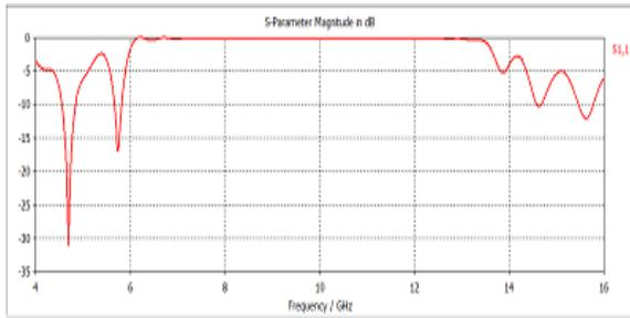
Fig. 2(a) Simulated S<sub>11</sub> parameter of EBG based Microstrip Filter Structure
