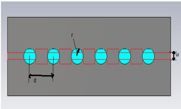
Fig. 1(b) Schematic of EBG based Microstrip Filter Structure (Bottom View)
