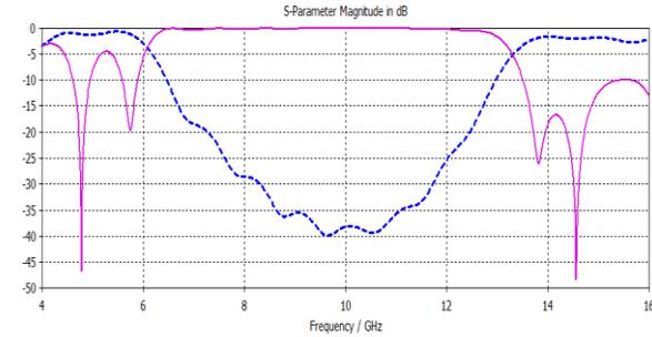
Fig. 4(a) Simulated  $S_{11}$  (solid line) and  $S_{21}$  (dotted line) for Triangular Window
