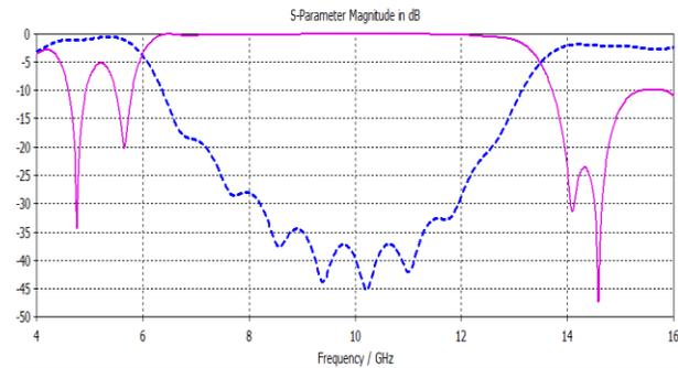
Fig. 4(c) Simulated  $S_{11}$  (solid line) and  $S_{21}$  (dotted line) for Hamming window
