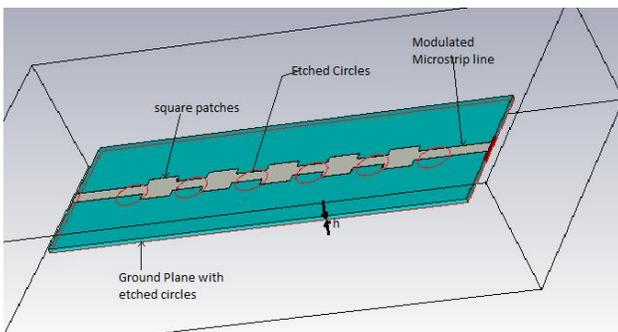
Fig. 1(c) Schematic of EBG base Microstrip Filter Structure (Side View)
