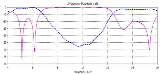
Fig. 4(g) Simulated  $S_{11}$  (solid line) and  $S_{21}$  (dotted line) for poisson window
