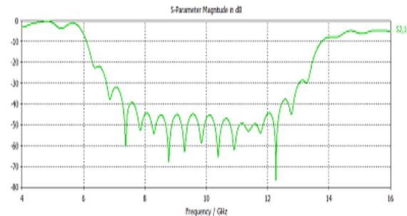
Fig. 2(b) Simulated S<sub>21</sub> parameter of EBG based Microstrip Filter Structure
