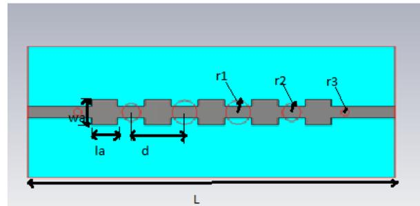
Fig. 3 Schematic of EBG based Microstrip Filter with Tapered Circles
