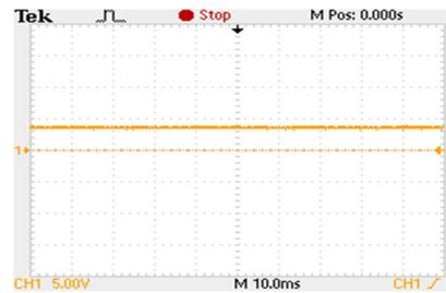
Fig.12 Output Voltage (+3.3V)
