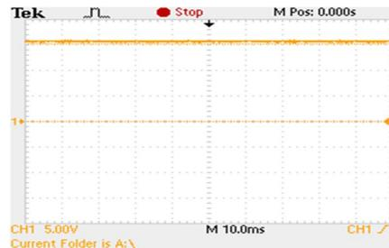
Fig.10 Output Voltage (+15V)
