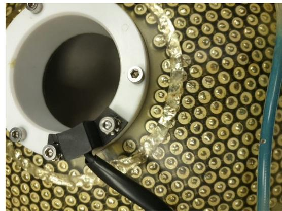
Fig. 9: Piezo emitters soldered to the base.
