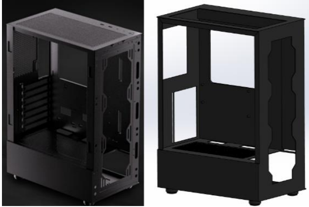
Fig. 1 Comparison between the real model and the model used for the simulations of the XPG VALOR AIR case
