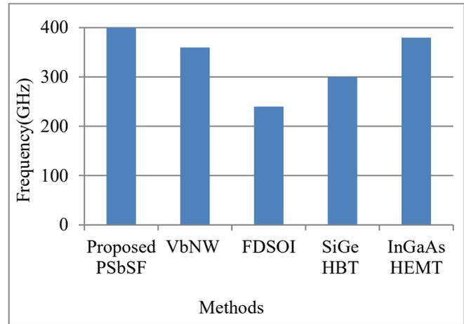
Fig. 22 Comparative of frequency for developed PSbSF-TCR
