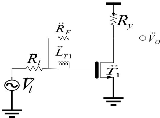
Fig. 5 Series resonators of LNA
