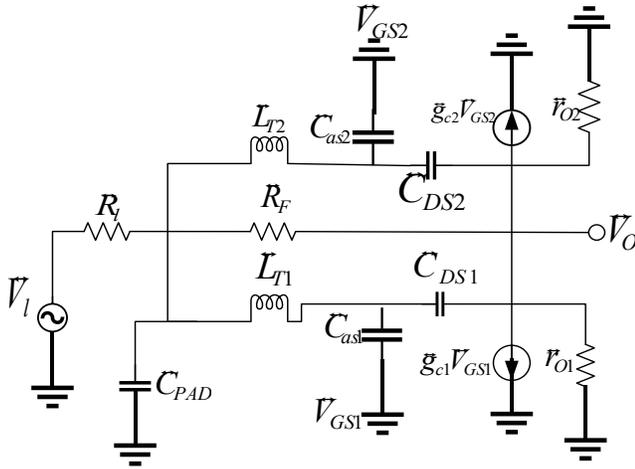
Fig. 7 Proposed modified shunt based resistive feedback
