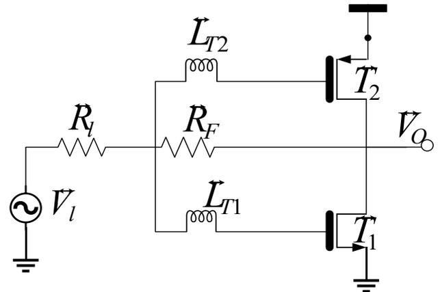
Fig. 6 Proposed shunt based resistive feedback
