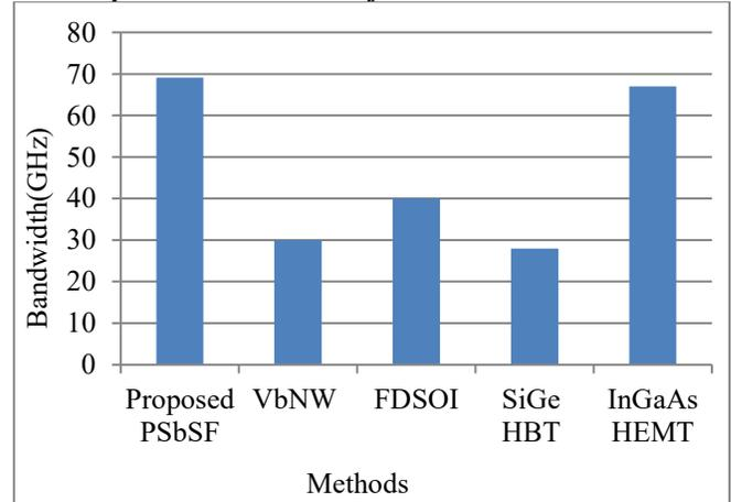
Fig. 18 Comparative of bandwidth for developed PSbSF-TCR
