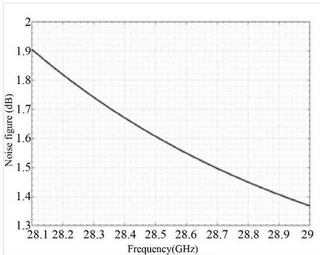
Fig. 10 Noise figure to the developed PSbSF-TCR
