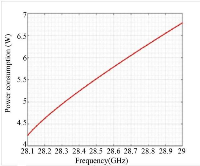
Fig. 9 Power consumption for developed PSbSF-TCR
