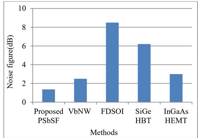
Fig. 17 Comparative on noise figure for developed PSbSF-TCR
