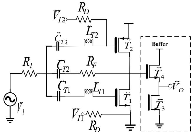
Fig. 3 Schematic diagram of proposed PSbSF-TCR topology
