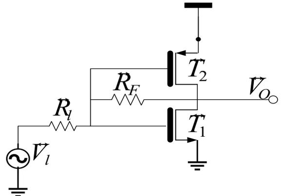
Fig. 4 Shunt-based resistive feedback to reuse current
