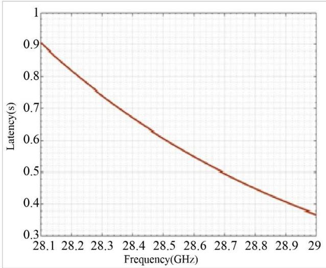
Fig. 12 Latency to the developed PSbSF-TCR
