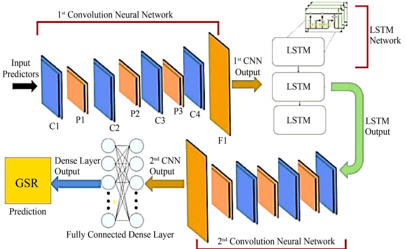
Fig. 3 Structure of the hybrid LSTM-GBM model
