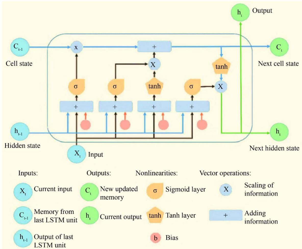
Fig. 1 Structure of the LSTM model
