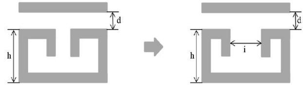
Fig. 2 Metamaterial structures with single-module acoustic pressure characteristics of the proposed methods
