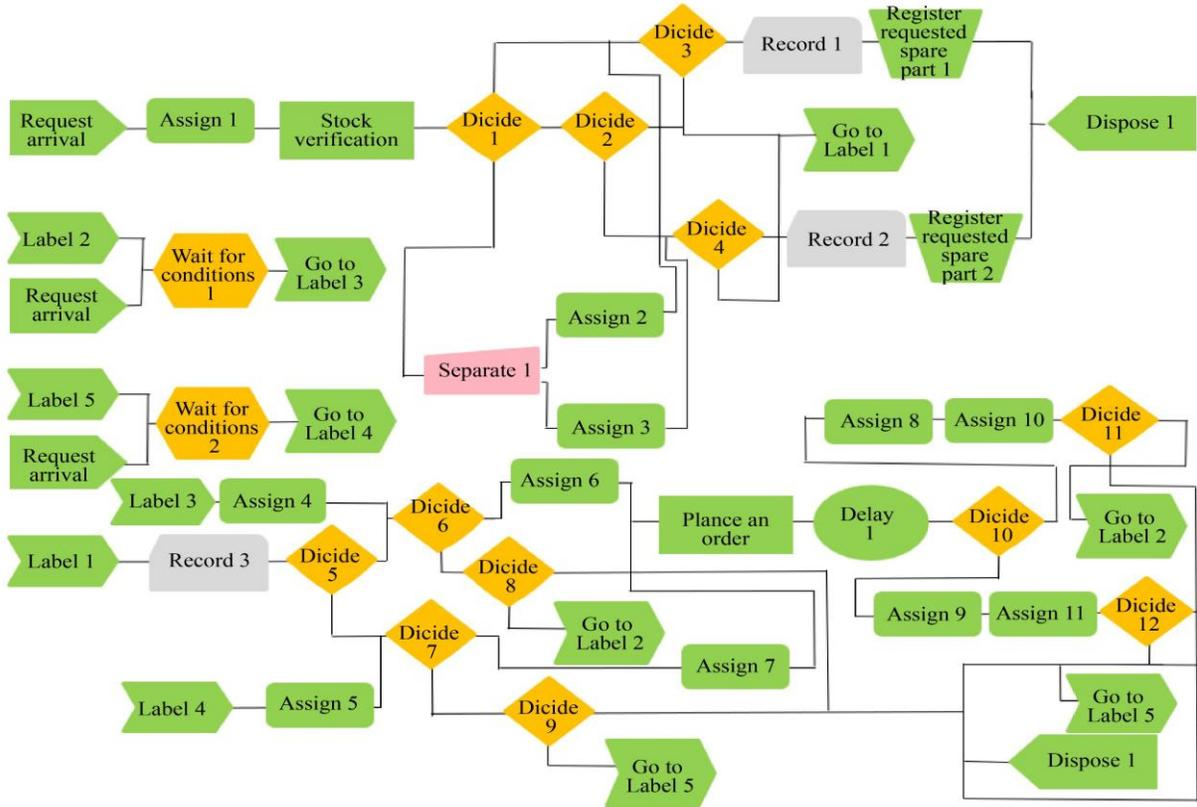
Fig. 10 Proposed model for the implementation of kanban tool in arena software
