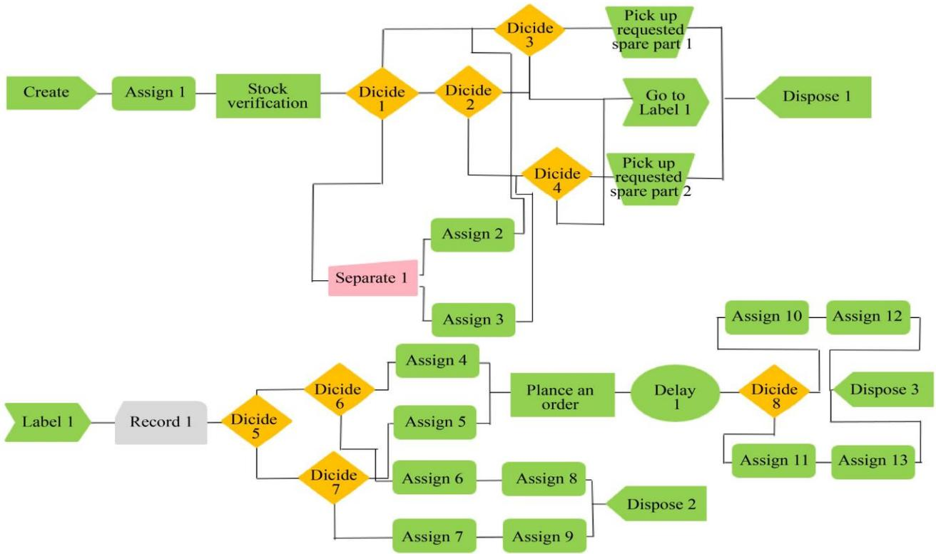
Fig. 9 Original model before the implementation of kanban tool in arena software
