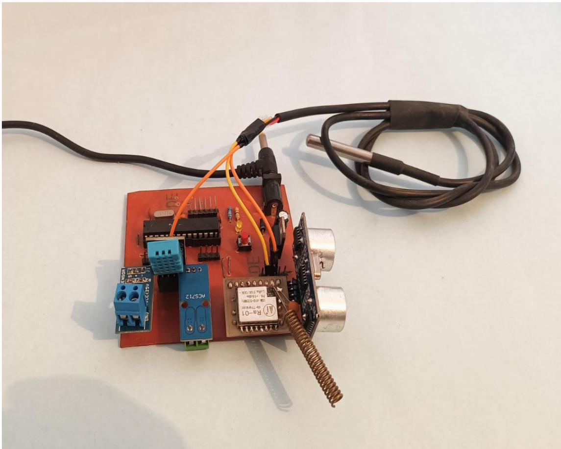
Fig. 5 Hardware node used for transformer health monitoring unit
