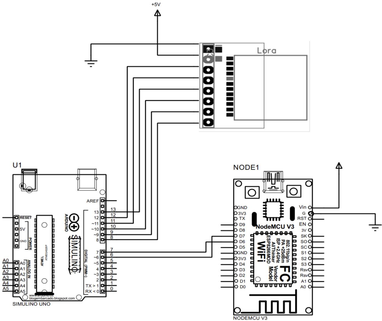
Fig. 4 Connection diagram of this edge gateway unit
