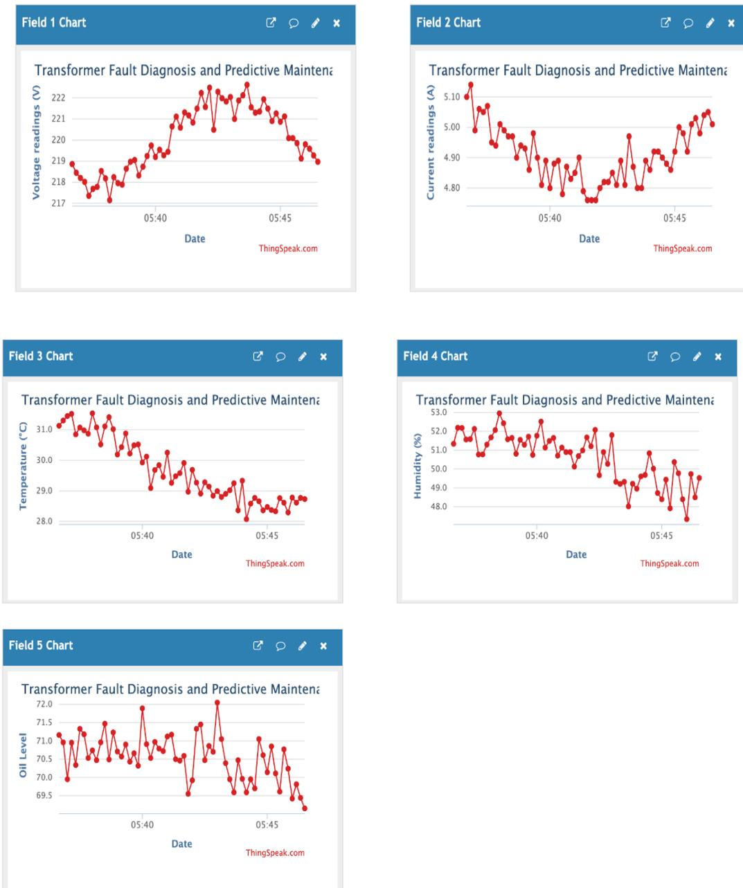
Fig. 7 Thingspeak web dashboard data visualization of the transformer health monitoring
