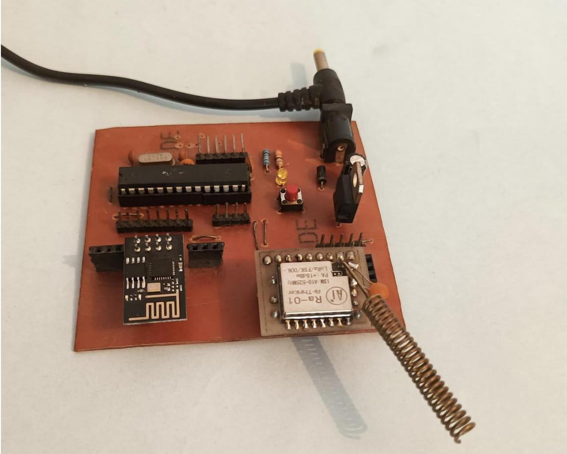
**Fig. 6 Hardware node used for edge gateway unit**
