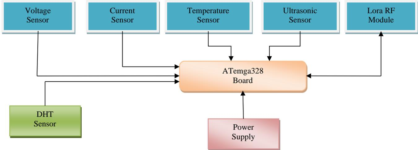
Fig. 1 Block diagram of the transformer health monitoring unit
