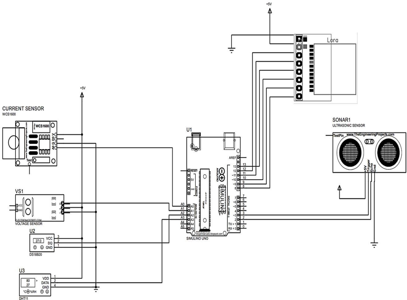
Fig. 3 Connection diagram of this transformer health monitoring unit
