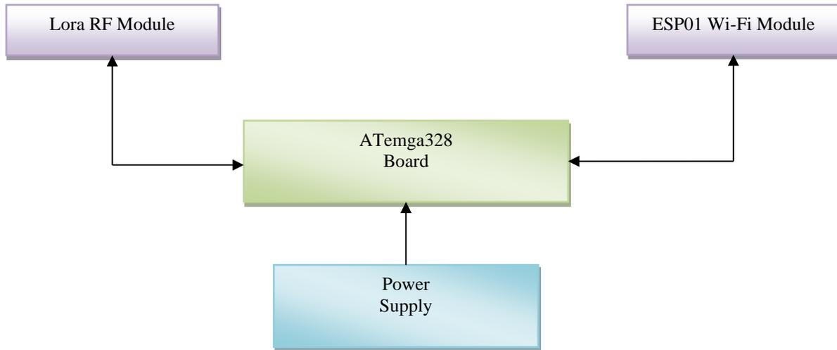
Fig. 2 Block diagram of edge gateway unit
