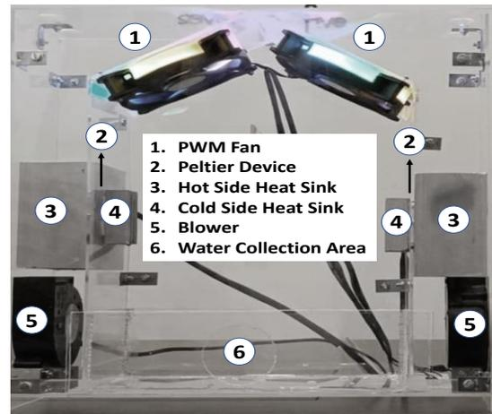
Fig. 7 Manufactured DCAWH
