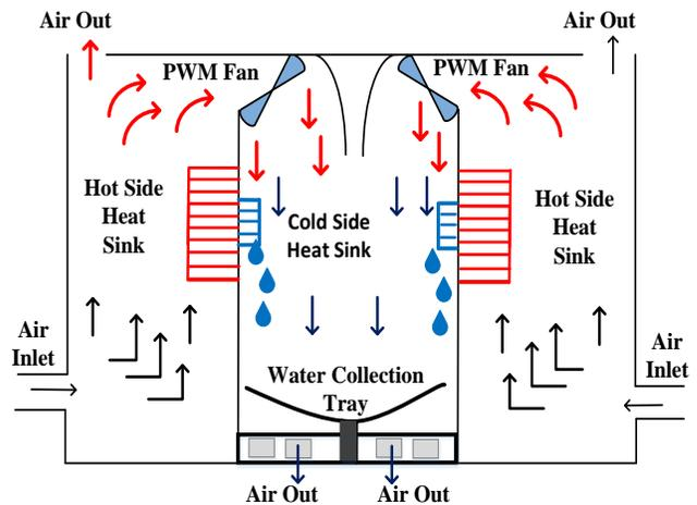
Fig. 3 Conceptual Diagram of Proposed Double Chamber Air Water Harvester (DCAWH). The harvester contains two Peltier modules, two pairs of heatsinks, two fans and two blowers.
