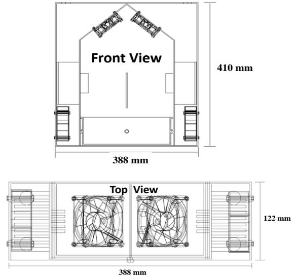
Fig. 6 2D views of proposed Air Water Harvester
