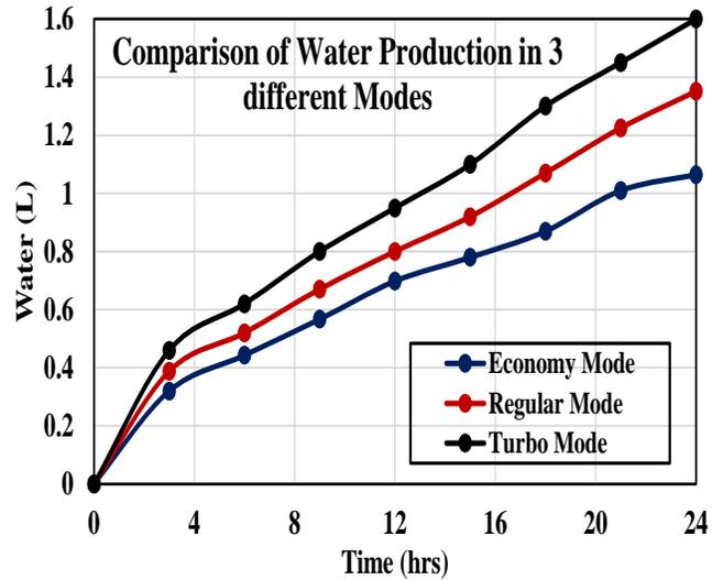
Fig. 12 Comparison of water production in three modes
