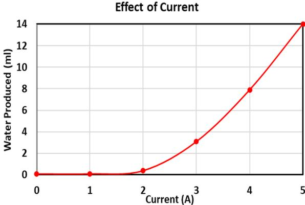
Fig. 8. Effect of current on water production
