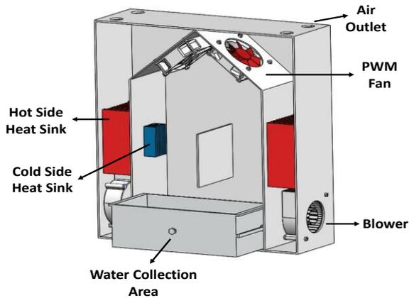
Fig. 5 3D CAD model of DCAWH
