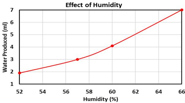
Fig. 9 Effect of humidity on water production
