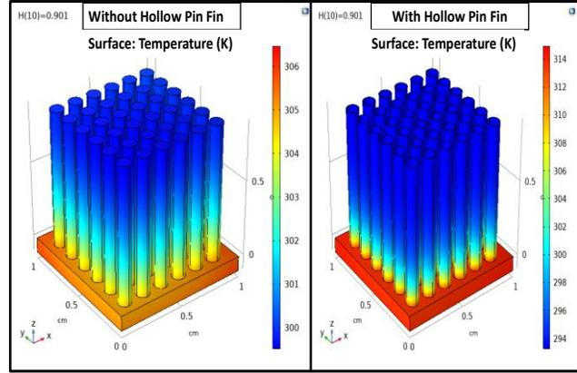
Fig. 10 Comparison of heat sinks in terms of heat dissipation
